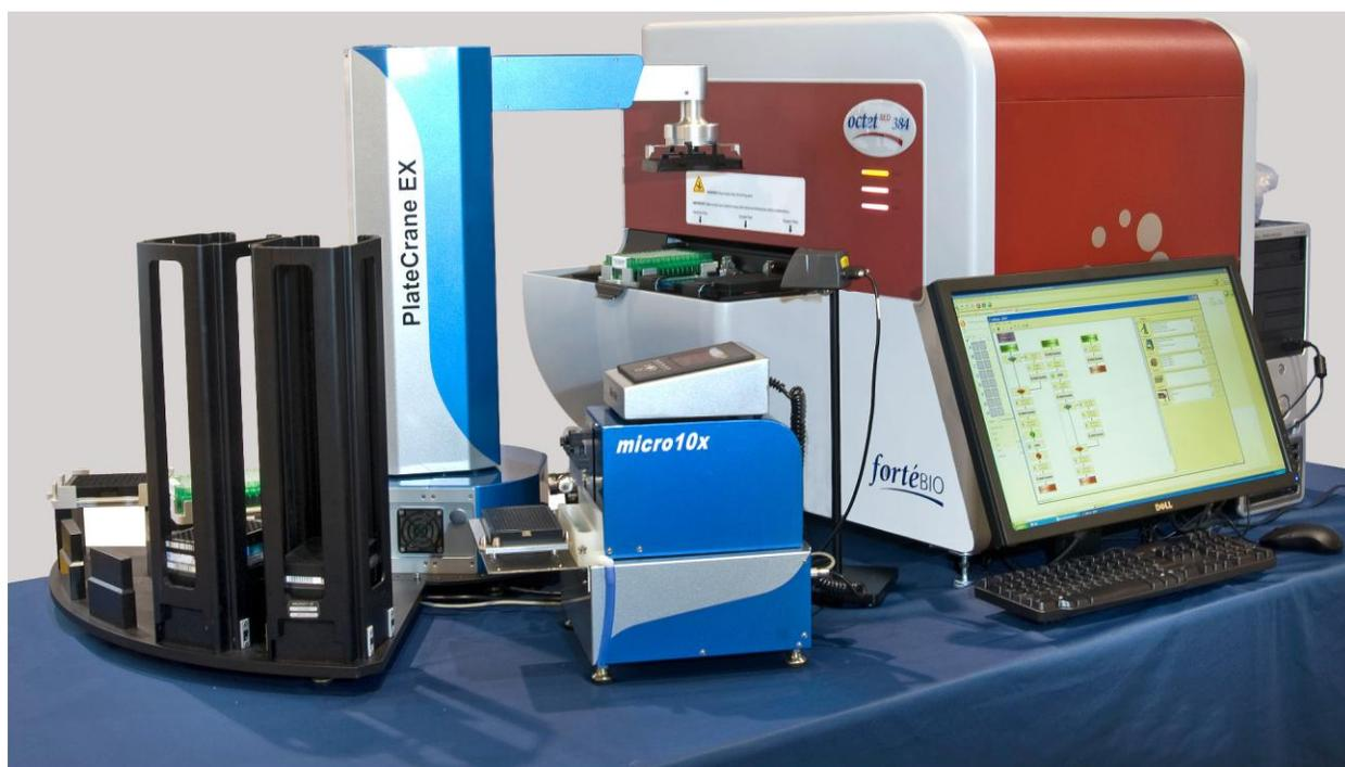
This workcell utilizes ForteBio's **Octet** platform that provides instruments, biosensors, reagents and assay kits for analyzing biomolecular interactions in 96- and 384-well microplate formats. The false readings, cost, and time associated with labeling are eliminated with the **Octet** platform which utilizes **BioLayer Interferometry (BLI)** technology.
